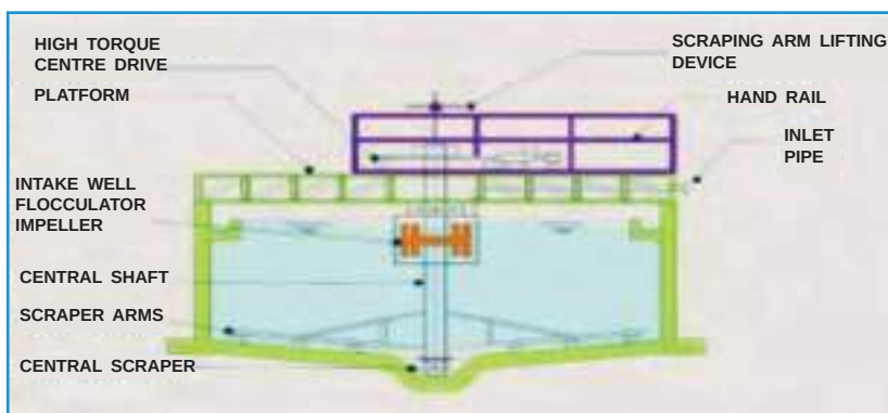
Fig 3.4 - General arrangement of clariflocculator
