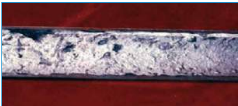
Fig 10.6 – Photograph of severely scaled boiler tube
