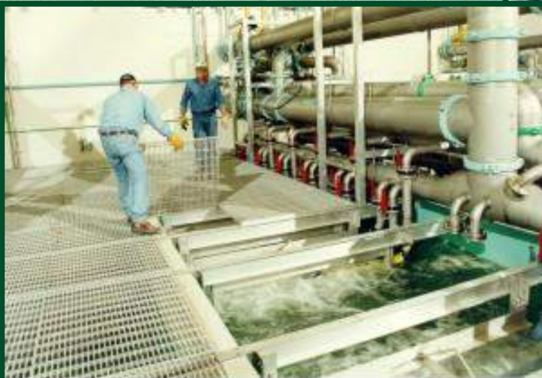
The ZeeWeed® membranes are immersed in the process tanks
