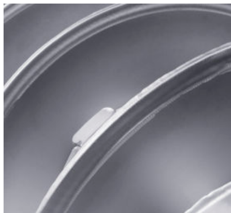
Figure 6. Flame sprayed tungsten carbide wear protection on conveyor flights
